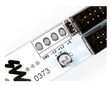
These connectors are provided for advanced users with sufficient knowledge of soldering and power systems. They can be used with a custom or specialized low-noise bus board system. While 4ms Company will warranty and support the internal circuitry of the **Row Power 35**, we do not offer support for 3rd party or DIY bus boards or distribution systems.
