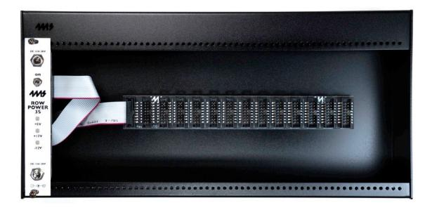
An example using a Bus Stick installed in a Pod64X is shown above. The Bus Stick can be secured to the case using the adhesive pads on the back. Make sure the surface is clean and apply pressure for 20 seconds. It's safe to daisy-chain a flying bus cable or another Bus Stick, but to insure the lowest noise system, use as few connectors as possible.
