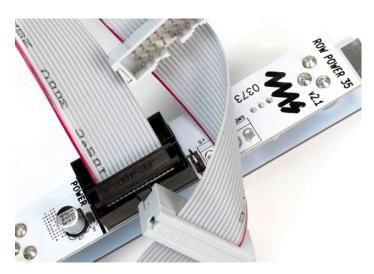
The **Row Power 35** can be used with flying bus cables, multi-power cables, bus boards and other passive distribution systems. There are two male pin headers on the back of the **Row Power 35**. You can use just one of the two headers, or both.
